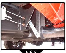
STEP 1 Remove front and rear body mount bolts. Replace with M12 & 4-3/4" bolt, lock washer, & flat washer supplied in the bracket kit. Adding the front and rear bracket under the lower body bushing and tighten these bolts to allow for minor adjustments. (Fig 1 thru 4) *On all 2006 and up models use factory body bolt. Making sure though to add 9/16" lock washer before replacing with bracket*
